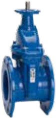
Series 15/42 Flanged gate valve with ISO top flange for actuator Face-to-face DIN F4 DN40-400 PN10/16 Ductile iron
