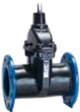
Series 02/52 Premium 100 gate valve Flanged Face-to-face DIN F5 DN40-500 Ductile iron External PUR coating
