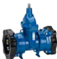
Series 636 Supa Maxi™ gate valve Universal and tensile coupling ends for all pipes Ductile iron DN80-300 PN16
