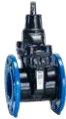
Series 06/52 Premium 100 gate valve Flanged Face-to-face DIN F4 DN40-600 Ductile iron External PUR coating
