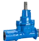
Series 03/40 Service connection valve for side tapping with internal thread /external thread DN25-50 PN16 Ductile iron
