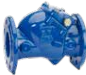
Series 41/61 Swing check valve Resilient seated Closed bushings DN50-300 PN10/16 Ductile iron
