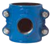
Series 10/00 Tapping saddle for uPVC and PE pipes DN50-300 Ductile iron Lower part in stainless steel from DN250
