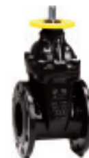
Series 15/78 Flanged gate valve with ISO top flange Short DIN F4 DN50-400 PN10/16 Ductile iron With external PUR coating
